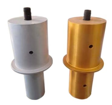
An ultrasonic booster is a mechanical device designed to increase the amplitude of ultrasonic vibrations generated by an ultrasonic transducer. It works by converting the low-amplitude, high-frequency vibrations produced by the transducer into higher-amplitude vibrations, which are then transmitted to the ultrasonic horn or sonotrode.
